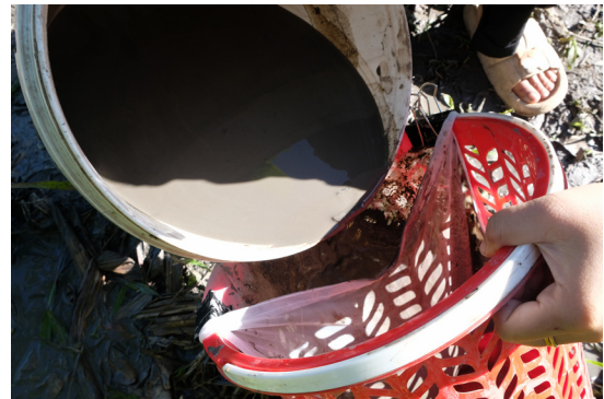
Fig. 6. Flotation method to collect the micro-materials.
