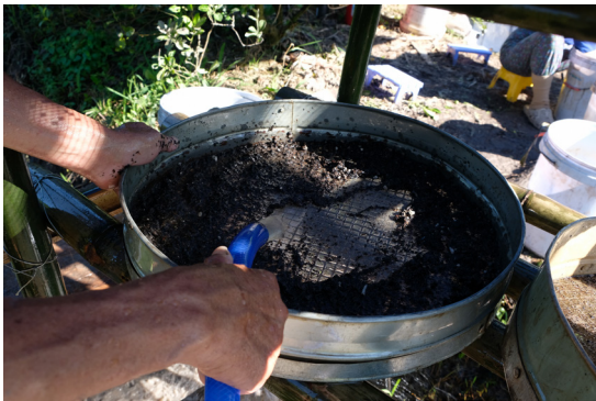
Fig. 5. Wet sieving method to collect the micro-materials.
